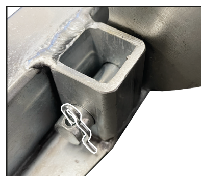
Fig. 4: Clevis pin secured using retaining clip
