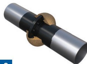
3 Denso Profiling Mastic or Densyl Mastic is applied
