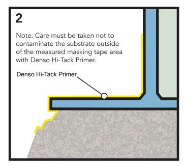
Measure, mask (50mm width masking tape) and prime the area for DENSO™ HI-TACK TAPE.
