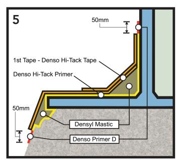
Measure and mask top and bottom allowing for the application of a 50mm strip of DENSO PRIMER  $D^{\text{TM}}$  as shown in red. Brush apply primer and allow to dry (approx 20 minutes). Now remove second two strips of 50mm width masking tape from top and bottom of application area.
