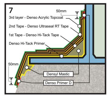
Brush apply 2 coats of the DENSO™ ACRYLIC TOPCOAT onto the DENSO ULTRASEAL RT TAPE.
