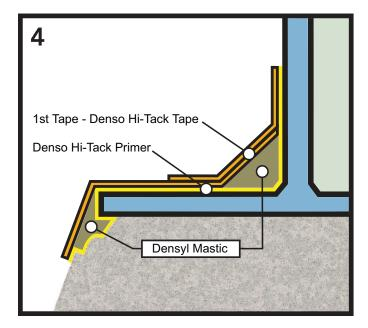
Apply the first strip of DENSO™ HI-TACK TAPE in line with the masking tape starting from the concrete base. Subsequent strips should overlap each other by a minimum of 50mm with the final strip applied in line with the masking tape on the vertical face. Smooth down all layers of tape ensuring there are no air pockets.
