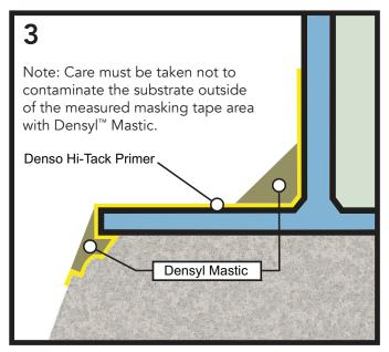
Fill all small voids, cracks and profile the 90° Tank Base angle with a 45° fillet of DENSYL MASTIC.
